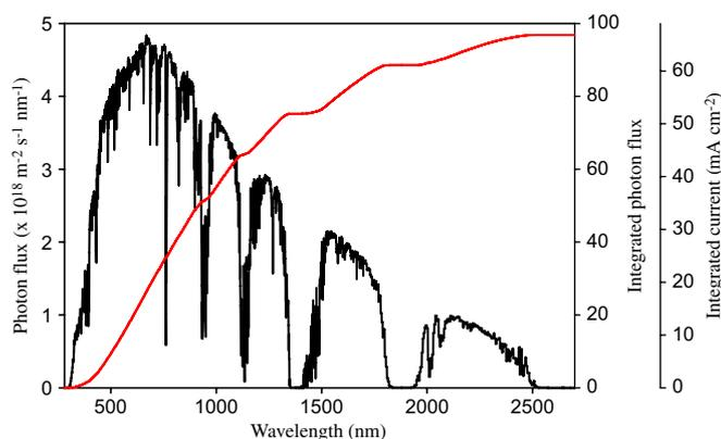
Fig. 1. Photon flux from the sun at the earth's surface ( $1000 \text{ W m}^{-2}$ , AM1.5G) as a function of wavelength. The integral of the curve is shown on the right y-axis as a percentage of the total number of photons and as the obtainable short circuit current density for an absorber material with a step function absorbance at that wavelength.
