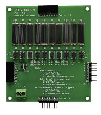
Each SolarBIT is connected to a 6-pin header. Using the included push-on shunts, the user can arrange the ten SolarBITs into various series/parallel combinations. To achieve maximum current, for example, all ten SolarBITs can be connected in parallel to yield 0.5 V at 400 mA. For maximum voltage, all ten SolarBITs can be connected in series to yield 5 V at 40 mA.
